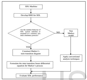
FIGURE 3 - Flowchart of reliability modelling of SDL by Markov Process
